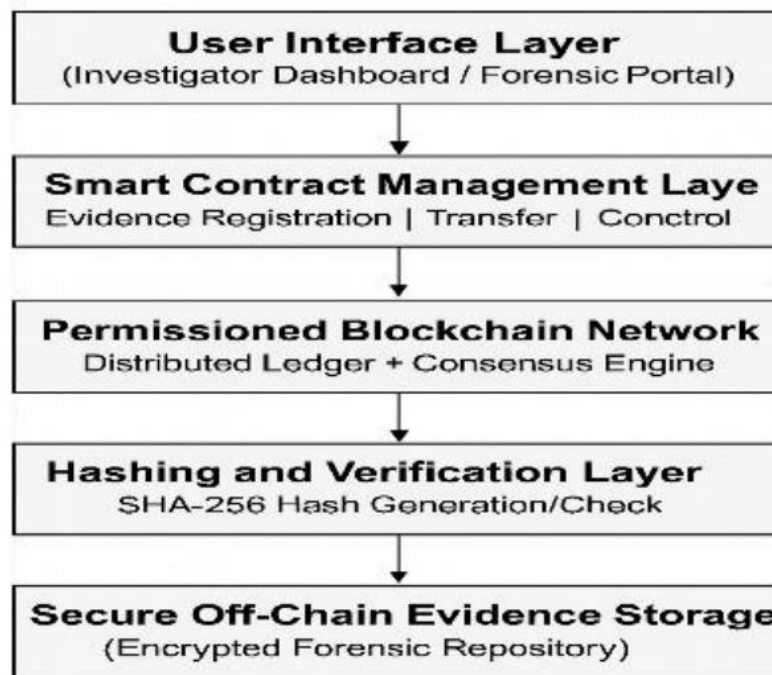
Fig. 2. Proposed blockchain-based chain of custody system architecture.
