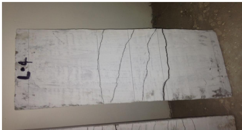
Fig 4.6: Crack Pattern for C-8 after testing up to Ultimate Load
