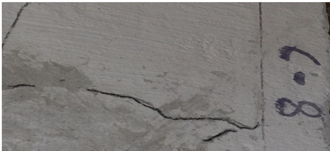
Fig 5.4 View of crack pattern under impact force of slab C-8
