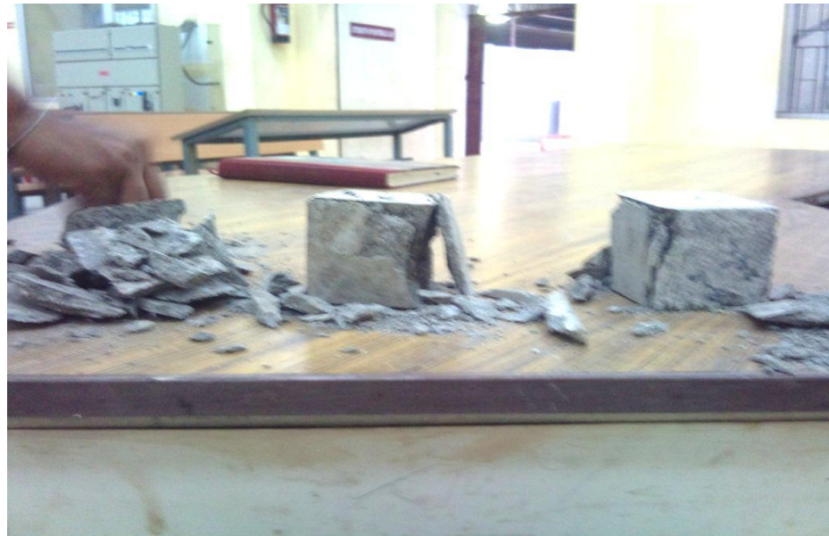
Fig 3.2: Failure Pattern of Cube after Ultimate Load
