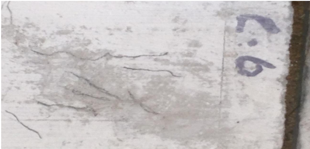
Fig 5.3 View of crack pattern under impact force of slab C-6
