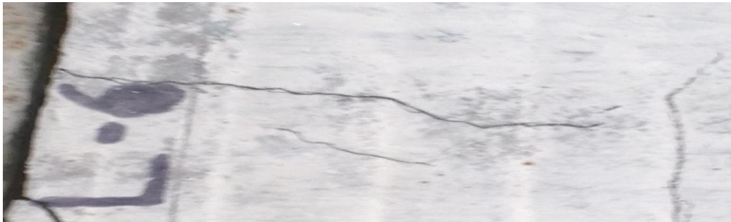
Fig 5.6 View of crack pattern under impact force of slab L-6
