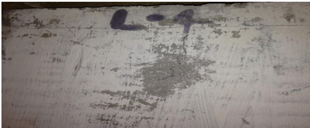
Fig 5.4 View of crack pattern under impact force of slab C-8
