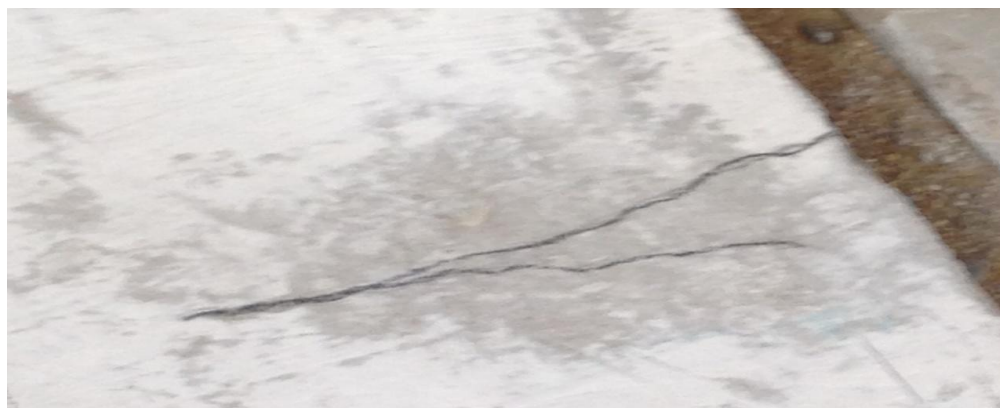
Fig 5.2 View of crack pattern under impact force of slab C-4
