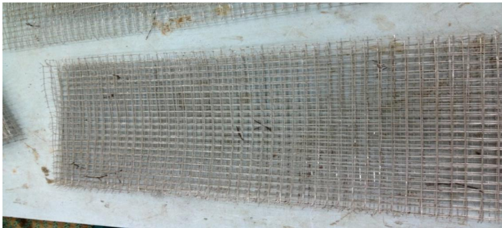
Fig 3.4 View of Square Welded Wire mesh Reinforcement Layers Using Binding Wires
