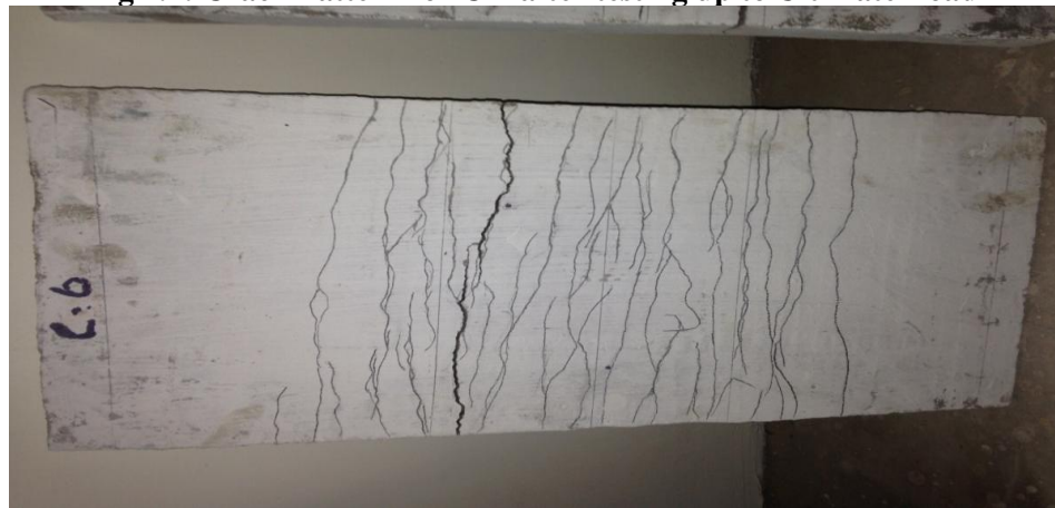
Fig 4.5: Crack Pattern for C-6 after testing up to Ultimate Load
