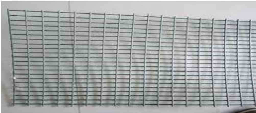
Fig 3.3 View of Square Welded Wire mesh Reinforcement
