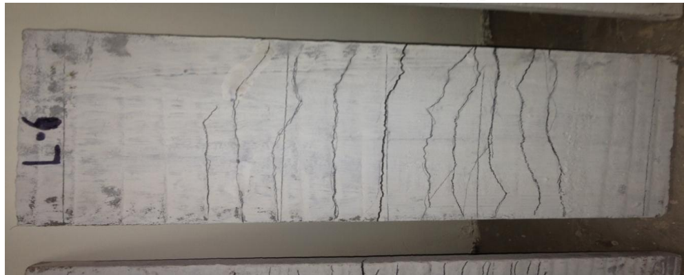
Fig 4.8: Crack Pattern for L-6 after testing up to Ultimate Load
