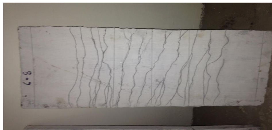
Fig 4.6: Crack Pattern for C-8 after testing up to Ultimate Load
