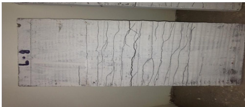
Fig 4.9: Crack Pattern for L-8 after testing up to Ultimate Load
