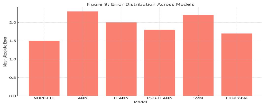
Here is **Figure 9: Error Distribution Across Models**. This bar chart displays the Mean Absolute Error (MAE) for different predictive models. It highlights that the NHPP-ELL model achieves the lowest error, with Ensemble and PSO-FLANN models performing comparably well. In contrast, standalone ANN and SVM show higher error, emphasizing the value of hybrid approaches.
