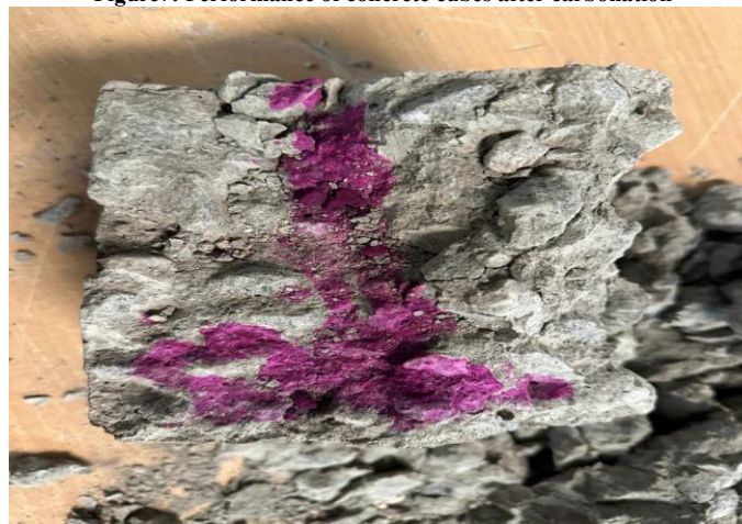
Figure 8: Concrete specimen subjected to carbonation
