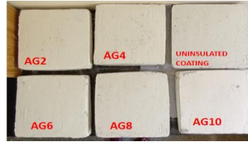
Fig.2: Experimental setup of thermal conductivity meter Fig.3: Aerogel coated thermal conductivity specimens
