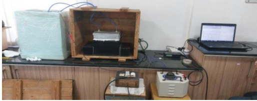
Fig.2: Experimental setup of thermal conductivity meter Fig.3: Aerogel coated thermal conductivity specimens
