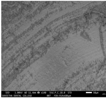
Figure 4: High-Magnification Morphological Characterization. High-resolution SEM image (1.90kx magnification) highlighting the micro-porous structure and surface roughness of the composite, which are critical factors for mesenchymal stem cell (MSC) attachment.
