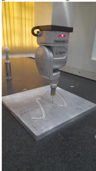
Fig 1 CMM Measurement of Profile Points
