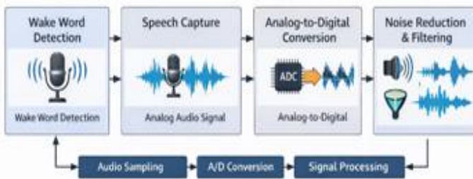
Figure 5: Voice Data Acquisition and Preprocessing Workflow for the Proposed AI Voice Assistant
