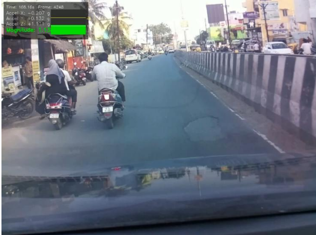
Fig. 2: Real-time road video feed showing the vehicle's perspective. The top-left overlay displays the accelerometer readings (X, Y, Z axes) and magnitude, which are used to detect vertical jolts indicative of potholes. This data is synchronized with the video frames for precise pothole detection.
