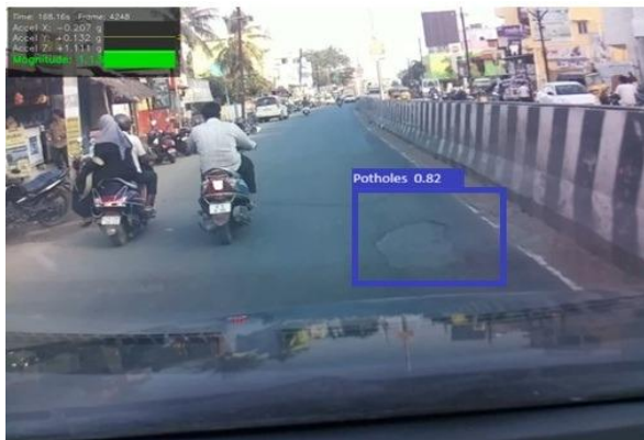
Fig. 3: YOLOv8 object detection results that highlights the potholes on the road's surface.
