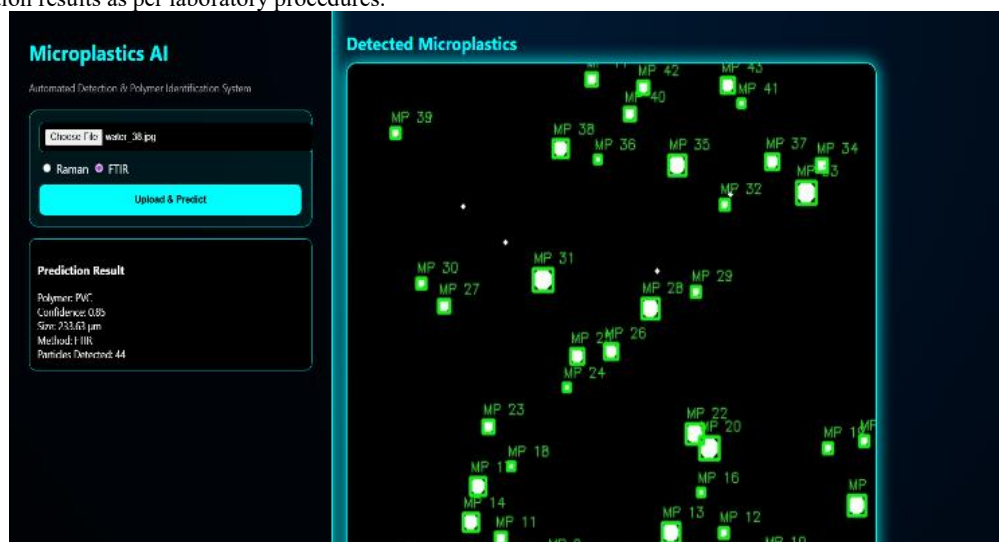
Figure 5.3. \mu\text{FTIR} -based microplastic detection and polymer prediction results with bounding boxes and particle labeling.
