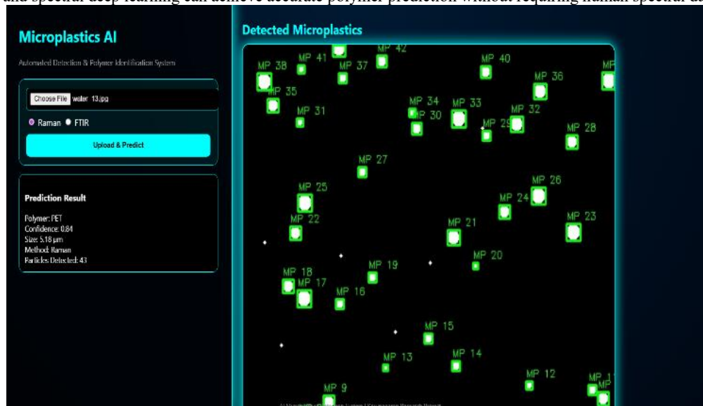
Figure 5.2. Raman-based microplastic detection and polymer prediction results with bounding boxes and particle labelling.
