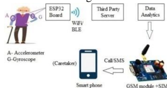
Fig. 1: System architecture of the EmoTrack wearable fall detection and alert framework. of data collection ensures comfort and long-term usability for elderly individuals.
