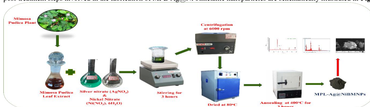
Figure 2. Schematic illustration of the green synthesis and post-treatment process for MPL–Ag@Ni bimetallic nanoparticles using Mimosa pudica leaf extract.
