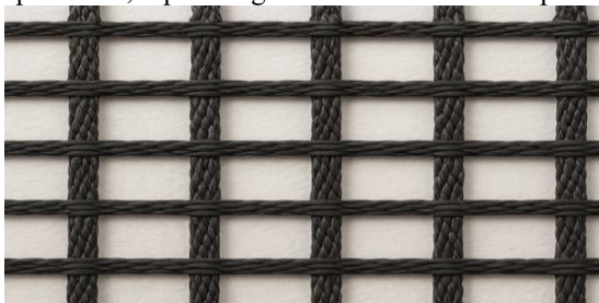
Fig 1. Close-up of basalt textile mesh
