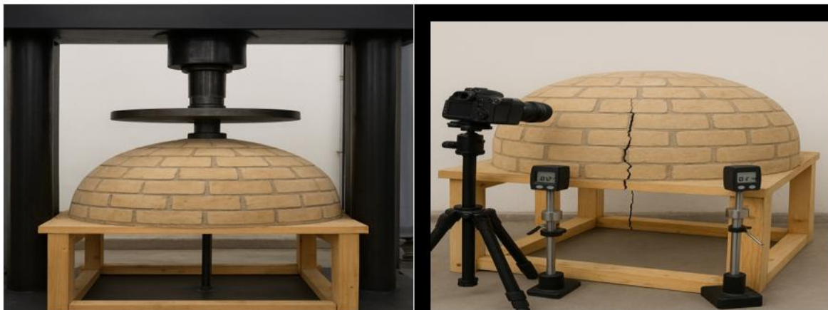
Fig6. Testing setup with load application at dome Crown & Crack monitoring setup (DIC cameras)
