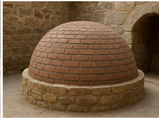
Fig4. Completed unstrengthened dome before retrofitting
