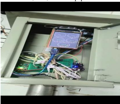
Figure 1. Sensor Device for Real Time Monitoring
