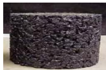
Fig 4.1: a)Marshall stability Specimen preparation b) Marshall stability Specimen
