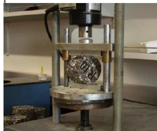
Fig. 4.6.: Indirect tensile strength test for BC mix Specimens
