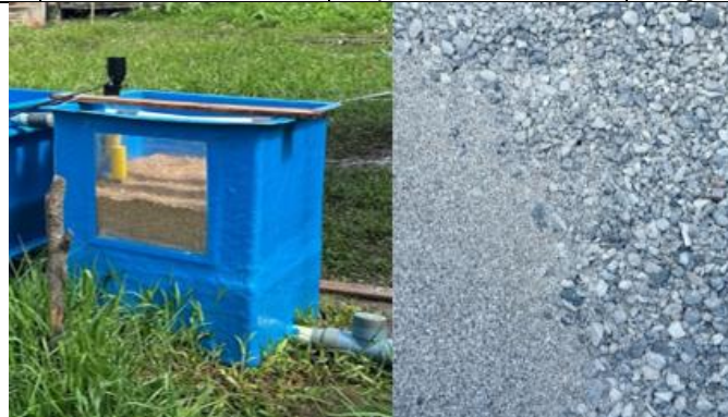
Fig 8. Filtration Unit and Filter Media
