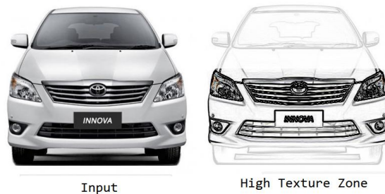
Figure 1: Input image and High-Texture zone extraction
