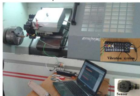
Figure 8 Machining setup with FFT analyzer setup. [29]
