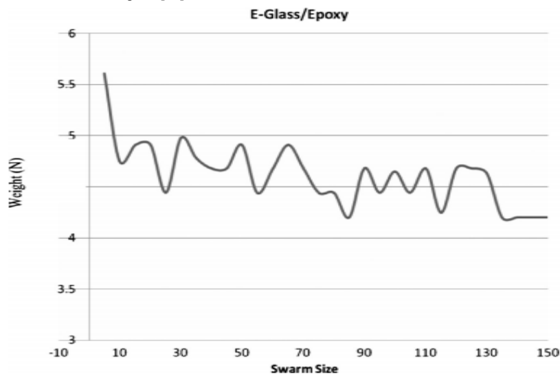
Figure 15 Variations of weight of E-Glass/Epoxy drive shafts with swarm size. [39]
