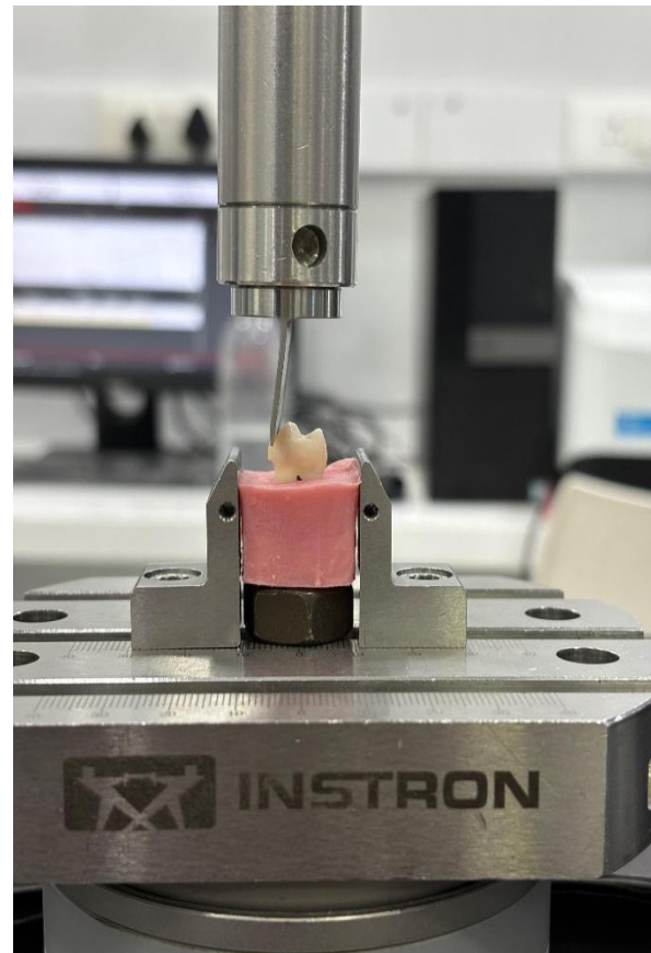
Image 2: Testing the shear bond strength of the sample.
