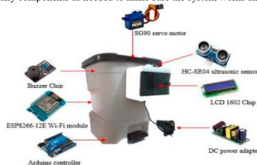
Figure 1: Smartbin Unit with Hardware
