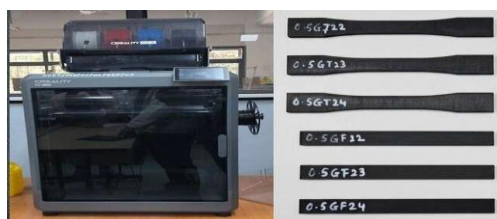
Figure 1: (a) ABS Creality K2 Plus 3D printer with multi-filament CFS unit; (b) ASTM D638/D7209 tensile specimens fabricated using graphene-reinforced
