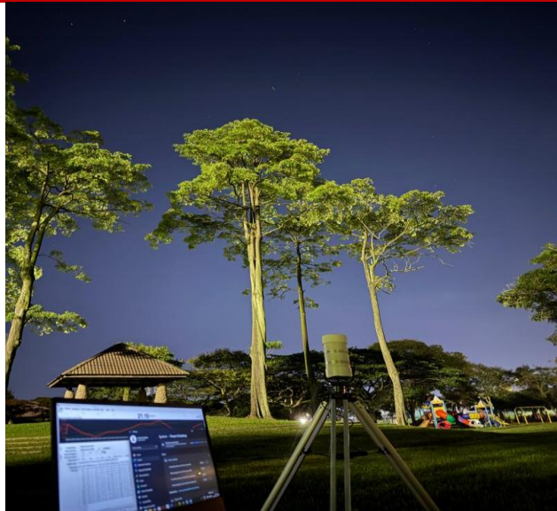
FIGURE 2. The Sky Quality Meter–LE (SQM-LE) was employed in this study to measure night sky brightness, expressed in magnitude per square arcsecond (mag/arcsec 2 ).
