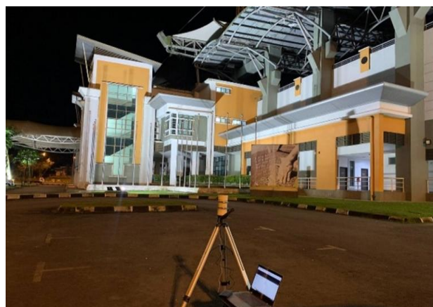
FIGURE 3 Night sky brightness was recorded using the SQM-LE installed on a tripod near a stadium with strong illumination, illustrating how nearby artificial lighting affects local sky conditions.
